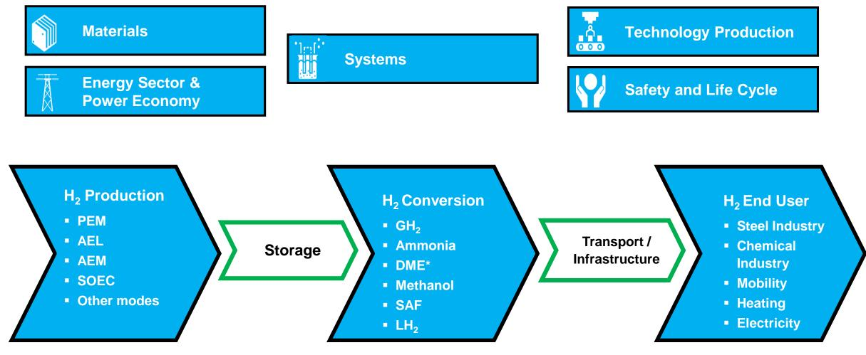
\*) Dimethyl Ether; H<sub>2</sub> carrier with high tech. storage capacity (26.1 wt%) compared to ammonia (17.8 wt%); methanol (18.8 wt%)
