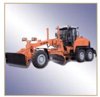
ON'S motor grader from 10 to 25t operating weight
